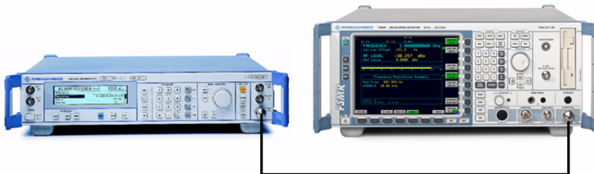
Fig.2-9 AM modulation measurement setup
