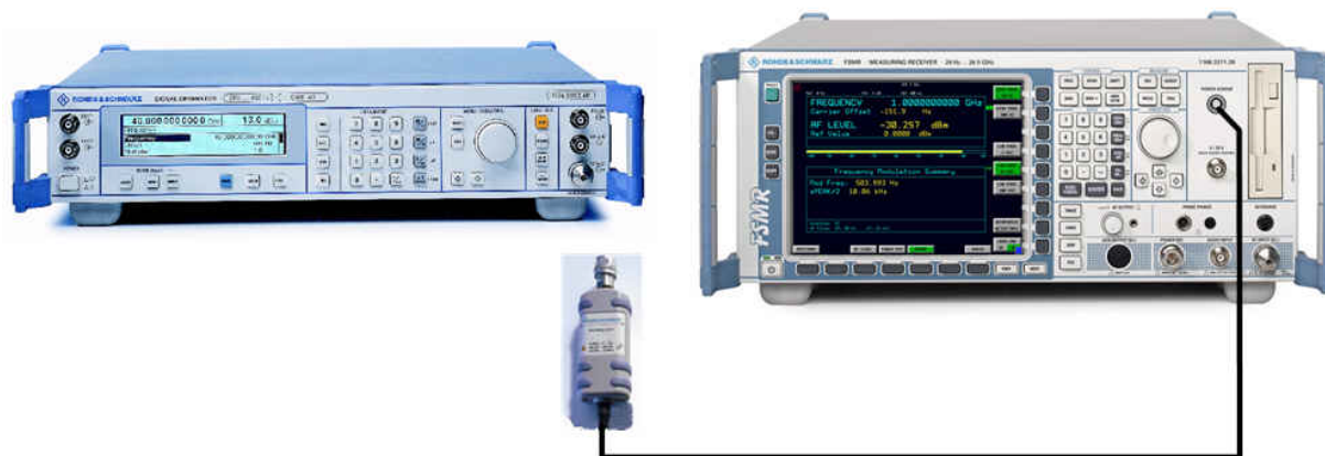
Fig.2-2 RF Power measurement setup
