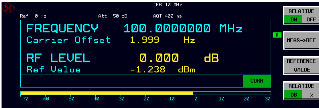
Fig. 4.4-5 Display mode for the relative level measurement RF Level
