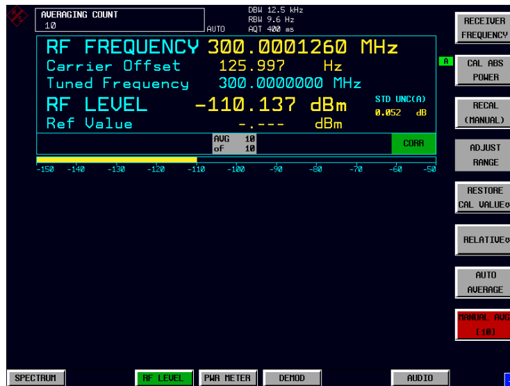
Fig.2-7 Tuned RF Level measurement at low levels
